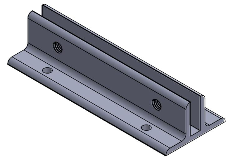
2 X M6x10mm set screw need to be install in the profile
